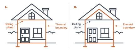
An example of a thermal boundary for a gable roof. House A has a vented attic with thermal boundary at the flat ceiling. House B is unvented with boundary at the roof line. (Source: Building Science Corporation (BSC))
