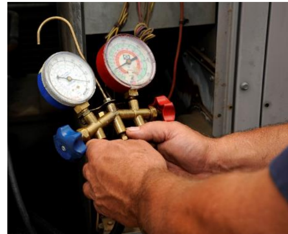
Refrigerant Gauges Not Connected
